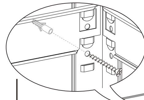
**EN** Move the rack to the desired place after finishing the assembly, then fix it to the wall with the anti-tipping devices to prevent any potential tipping hazards caused by uneven ground or unevenly distributed items.
