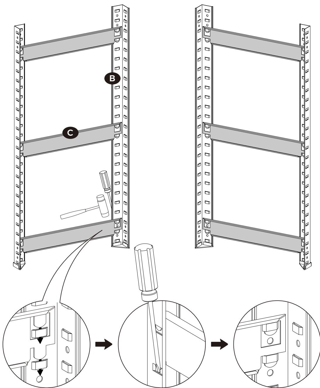
**EN** Insert both of the part C clips into the two slots of part B and make sure both of the clips pass entirely through the slot with its tip coming back out to the front to form a firm joint.
